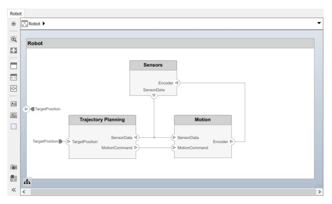
The architecture itself can also have ports. In this example, the target position for the robot is provided by a computer, external to the robot architecture. Represent this with a port on the architecture. Click the left edge of the architecture and type the port name TargetPosition.
