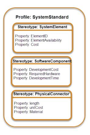
Each profile comes with a set of stereotypes, and each stereotype comes with a set of properties.
