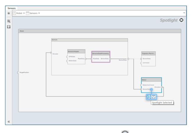
Return to the architecture model view by clicking the icon. To view the architecture at the level of a particular component, select the component and click the 📰 icon.
