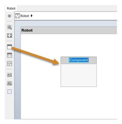
Type the name of the component, Sensors, in the text box that becomes active. Also add a Motion and a Controller component. Component names must be proper variable names. Click components and drag them to move to complete the layout.
