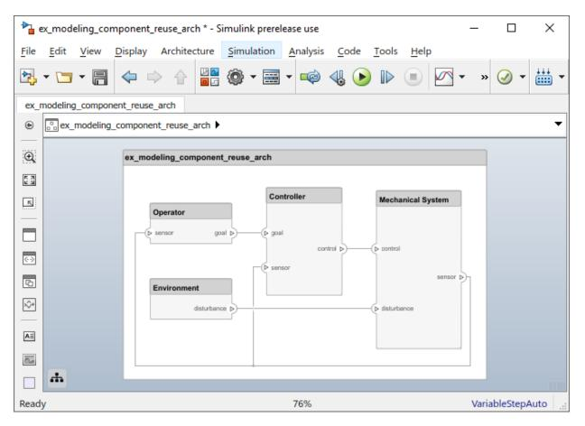
Each subsystem in the Simulink model corresponds to a component in the architecture model so that the hierarchy in the architecture model reflects the hierarchy of the behavior model.
