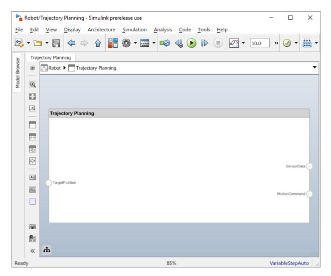
This component first computes an ideal position and velocity command using the motor position data that is part of the SensorData interface, and then uses the obstacle proximity information from the same interface to condition this motion command according to some safety rules. Add Motion control and Safety rules components as part
