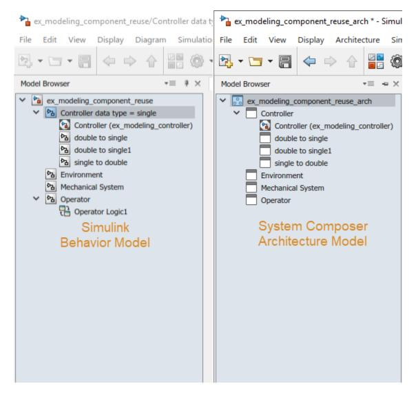
The requirements for subsystems and Model blocks in the Simulink model are preserved in the architecture model.
