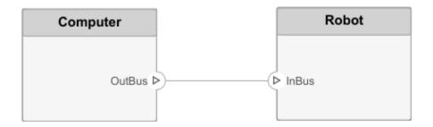
You can write an interface to fully specify a connection (and its associated ports). An interface can consist of multiple data elements with various dimensions, units, data types, etc. You can also associate interfaces with unconnected ports during component design, to enable consistency checking when connecting that port.
