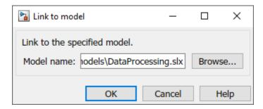
Any subcomponents and ports that are present in the components get deleted when the component links to a Simulink model.
