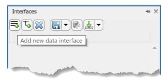
Type in the name of the interface, sensordata. Add an element to the selected interface: Click To and type timestamp.
