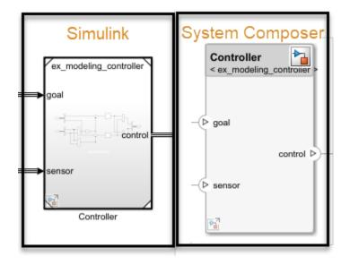
Buses at subsystem and Model block ports, as well as their dictionary links are preserved in the architecture model.
