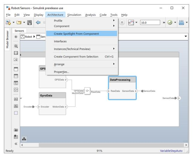
The spotlight view launches and shows all model elements to which the DataProcessingcomponent connects. The spotlight diagram is laid out automatically and cannot be edited.
