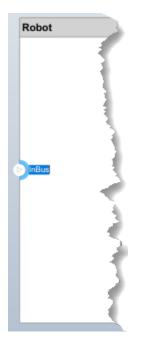
You can connect an architecture port to a component by dragging a line. Connections to or from an architecture port appear as tags.
