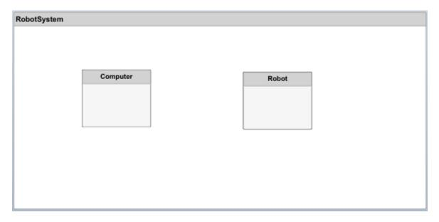
You can add non-visual properties to a component to capture its specifications relevant to the problem at hand. For example, if the total power consumption of the system is a concern, a Power Consumption property is necessary. You can add this property to a component using an "electrical component" stereotype.
